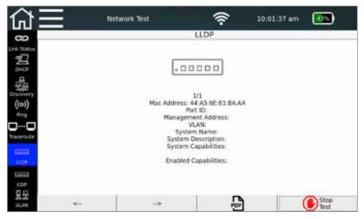
Detects Cisco Discovery Protocol (CDP) or Link Layer Discovery Protocol (LLDP) and displays information from the switch.
